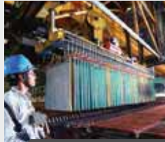
Cathode plates at Refinery cell house, Sterlite Tuticorin
