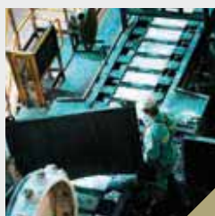
Ingot casting line at Skorpion integrated zinc complex
