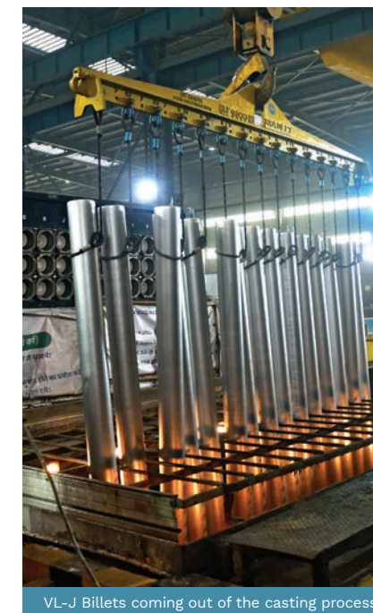
VL-J Billets coming out of the casting process
