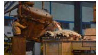
Above: Alumina refinery, Lanjigarh Below: Molten aluminium being poured in the smelter, Jharsuguda
