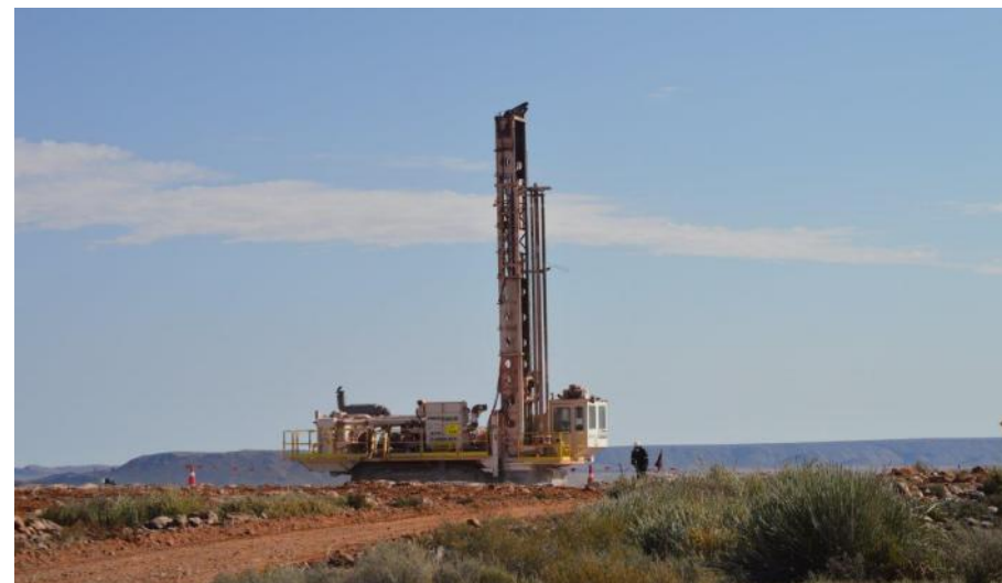
Blast haul drilling at the greater Gamsberg area
